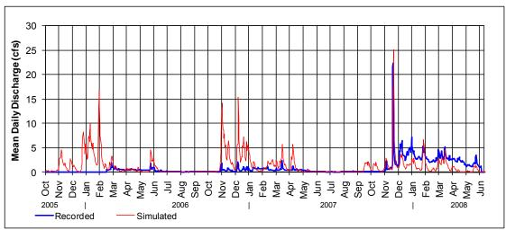
Figure 8 – Comparison of Simulated and Recorded Flow at Mouth of Ebright Creek (Note: Gage not used for Calibration due to data Quality Concerns)
