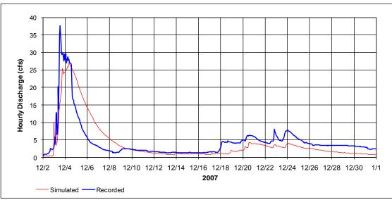
Figure 9 – Comparison of Simulated and Recorded Flow at Mouth of Ebright Creek December 2007 Storm
