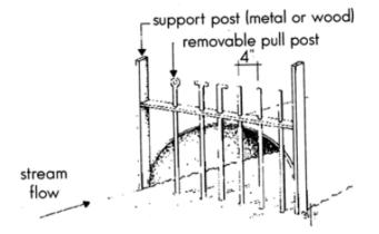
3. **Culvert Protector/Cleaner**: This alternative is similar to the Removable Pull Rod Grill, with the exception that the logging chain located at the top of the culvert is hooked to the bumper of a truck in order to lift the culvert cleaner out of the water to maintain and clean.
