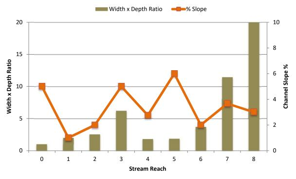
Figure 3: Width-to-depth Ratio and Stream Channel Slope for Each Reach Section
