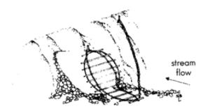
4. **Vertical Cylindrical Wire Mesh Beaver Guard**: This alternative protects the culvert inlet with a larger surface area than the previous two alternatives. The larger the wire mesh, the less maintenance needed to clear the debris.
