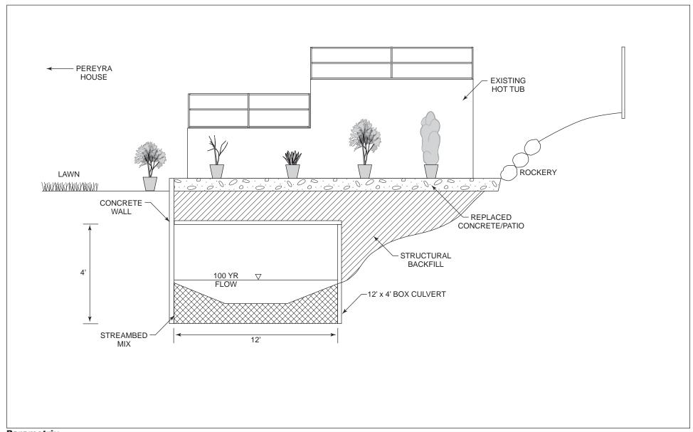
Figure Culv-1(c) Cross Section View Upstream of Culvert NTS
